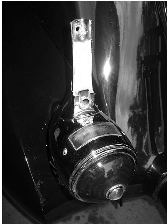
The epoxy repair will be hidden by the license plate.
