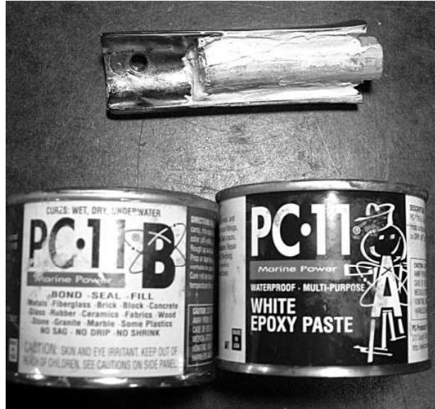
Two-part epoxy bonds the dowel to the broken piece.
