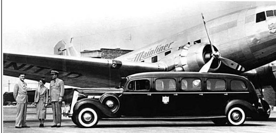
This is a '37 120 8-door airport limo, on an extended wheelbase, parked by a period United Airlines Mainliner. Looks like a posed publicity shot. A few of these stretch-jobs have survived.
