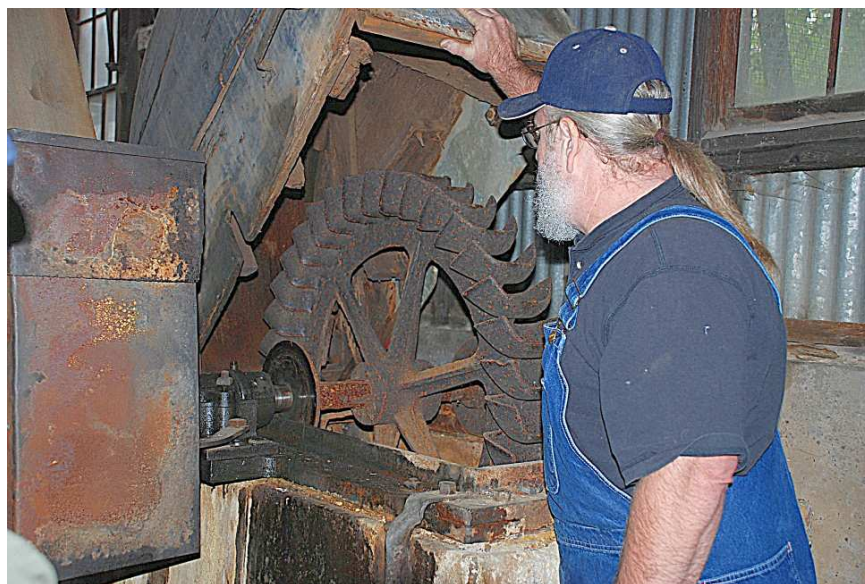
At the Knight Foundry in Sutter Creek, our guide showed us the original Knight Wheel that had cups that were hit by a stream of water that turned the wheel and powered the entire shop.
